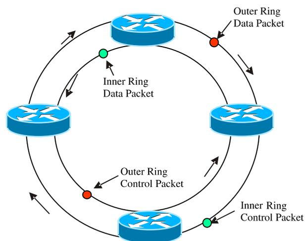
The RPR, being a Layer-2 network protocol, the MAC layer contains much of the functionality for the RPR network. The RPR MAC is responsible for providing access to the fibre media. The RPR MAC can receive, transit and transmit packets.
