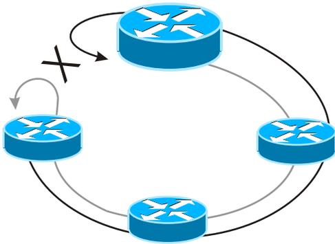
Regardless of the protection mechanism used, the ring will be protected within 50 ms.
