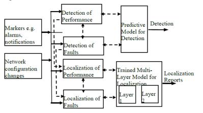
Fig 2. Fault/Performance Detection and Localization Model
