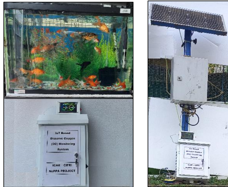
Fig 5 IoT system deployed in the aquarium and pond system
