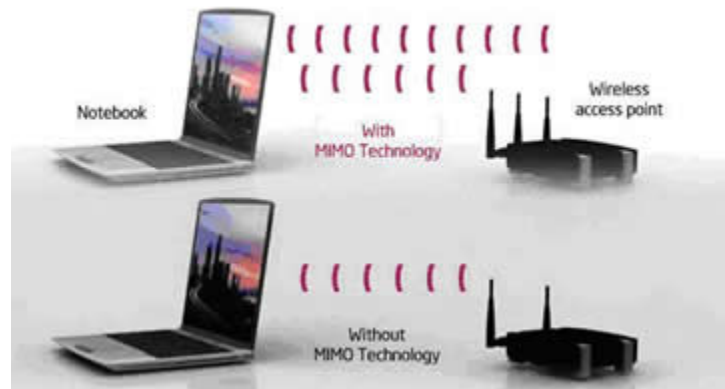
Figure-1 : MIMO Technology uses multiple radios to transfer more data at the same time
