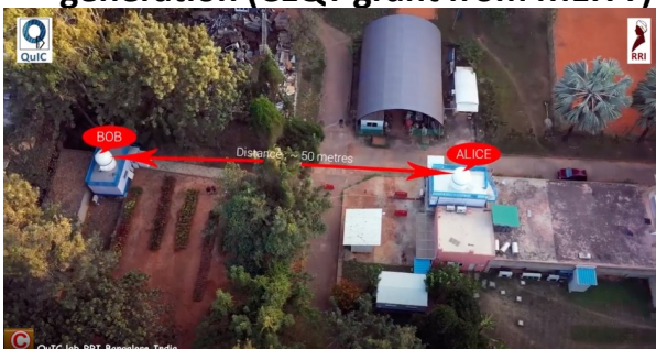
First demonstration of quantum key distribution between two buildings using an atmospheric free space channel in India (February 2022).
