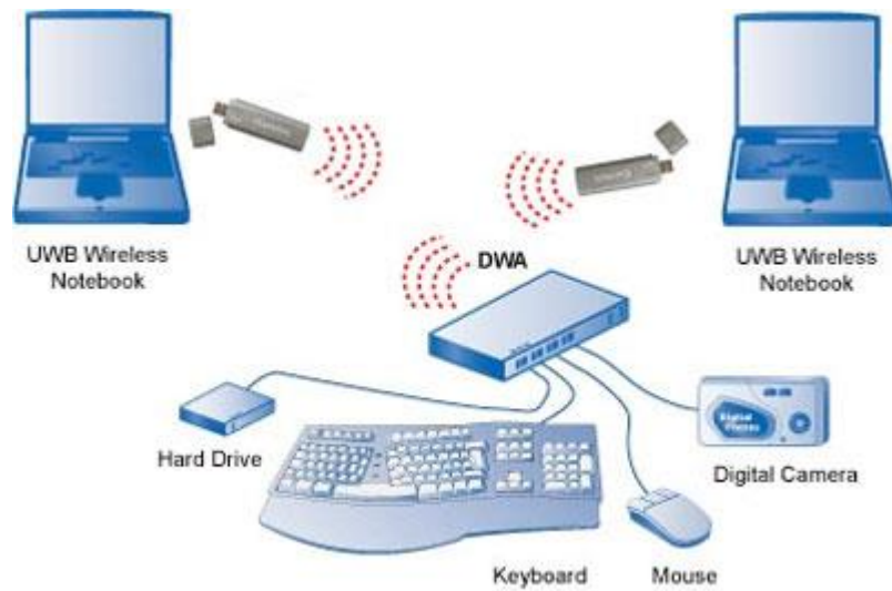
Figure 20 : Wireless USB Supporting Cluster Connectivity, [13]
