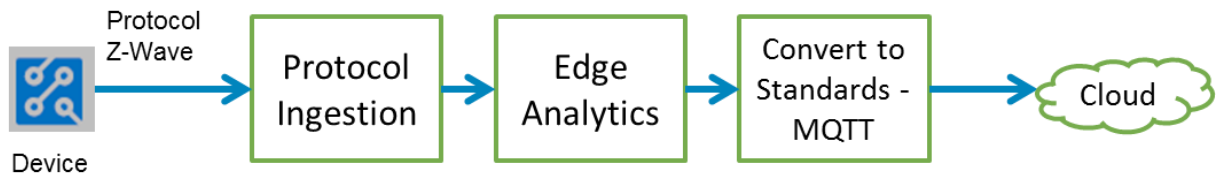
Figure 21 : Z Wave Architecture
