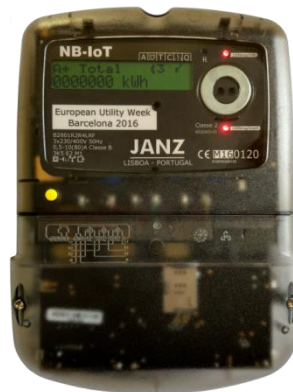
Fig ANNEX2.1: Energy Meter [A2.5]
