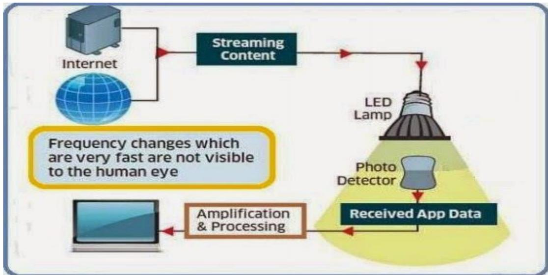
Fig 6: Block diagram of Li-Fi Sub System
