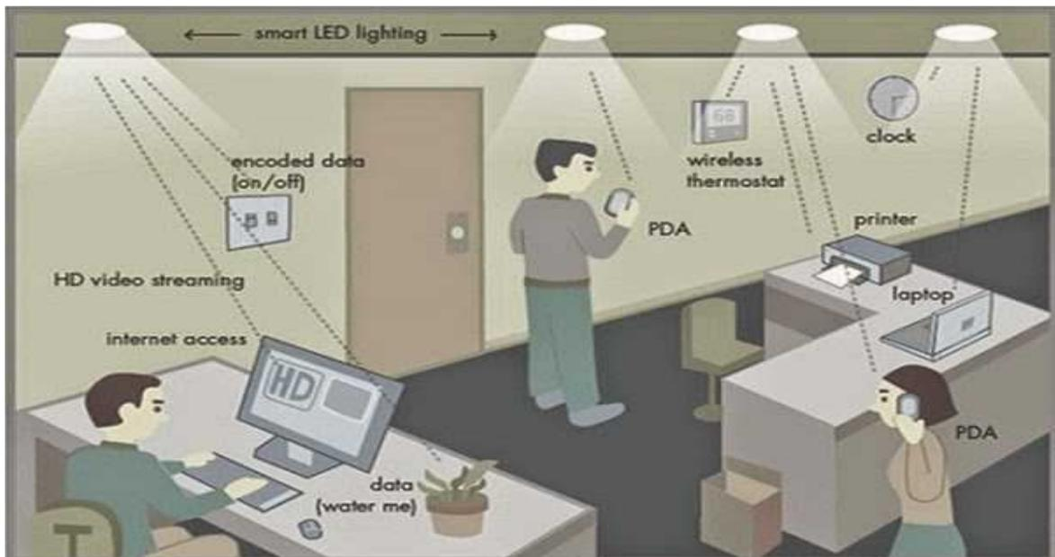
Fig 7: Li-Fi system connecting devices in a room
