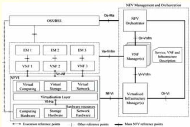
**Fig. 2: NFV reference architecture framework**
