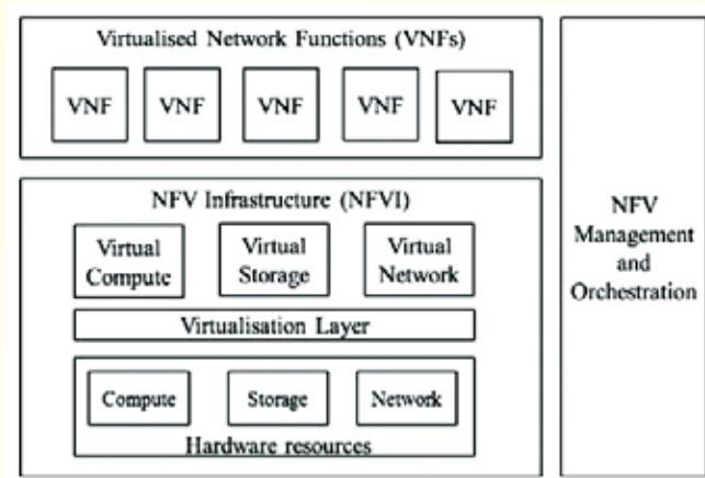
**Fig. 1: High Level NFV Framework**
