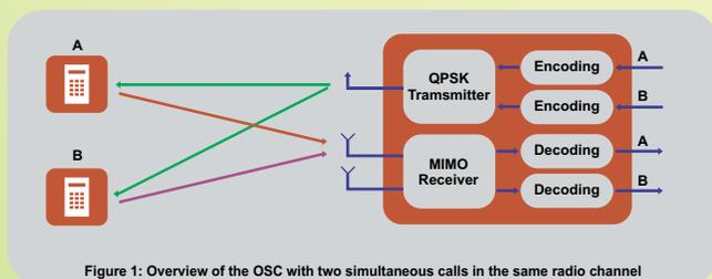
Figure 1: Overview of the OSC with two simultaneous calls in the same radio channel
