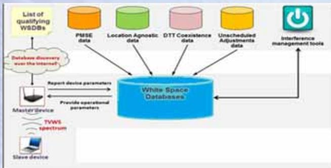
**Figure 1: Typical implementation of Geolocation Database based TVWS technology**
